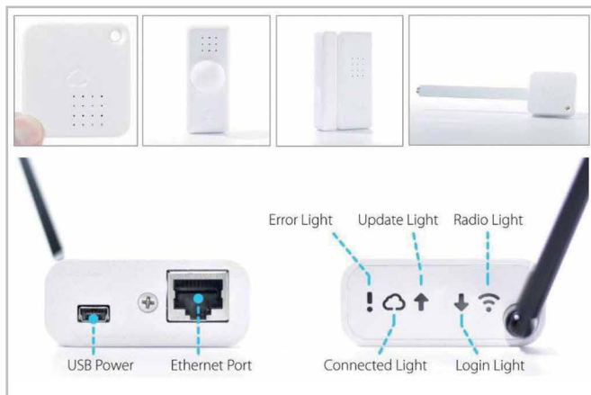
Figures 1a-e My Wireless Tag sensors and gateway device
