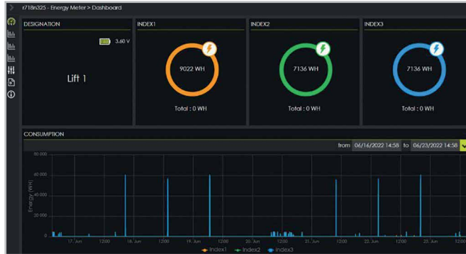
Figure 9 ALLIoT Energy Meter Dashboard Example
