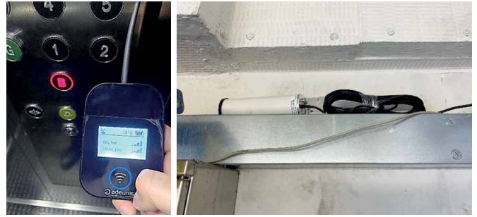
Figures 6a&b ALLIoT field test device and antenna extension
