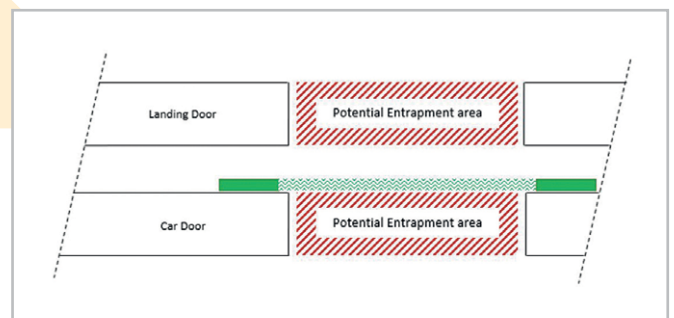
Figure 3: Overhead view diagram of lift door 'light curtain' with common mounting position (indicated green)
