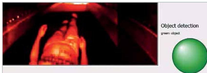
(b) One person is detected during entering the lift
