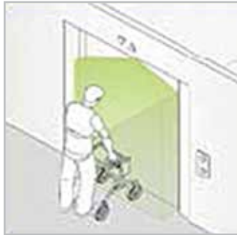
Figure 11 Full door area safeguarding with a 3D ToF sensor
