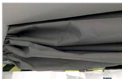
Fig. 5 Photo showing the most common headache – jamming in the side guides.
