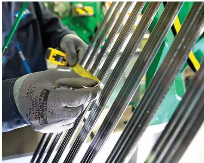
Figure 6. KONE UltraRope is made of carbon fiber, reducing cable weight by up to 80 percent. © KONE
