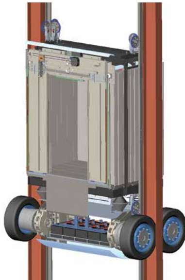
Figure 9. Otis ropeless elevator concept. © Otis Elevator Company
