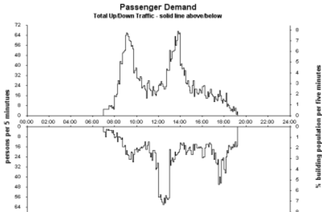
Figure 6 Graphical Representation of traffic over a whole day in a sample multi-tenant office building
